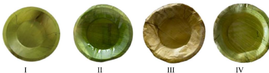
Fig. 2 Appearance of hyacinth leaf plates. I: without extraction, II: with simulant A, 10% ethanol, III: with simulant B, 3% acetic acid, IV: with simulant D2, isooctane.
