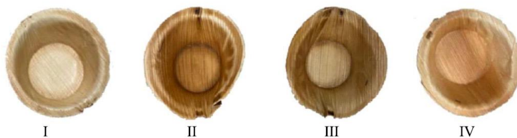
Fig. 3 Appearance of areca leaf plates. I: without extraction, II: with simulant A, 10% ethanol, III: with simulant B, 3% acetic acid, IV: with simulant D2, isooctane.
